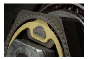
Retainer Tab secured in groove (FF Style).
